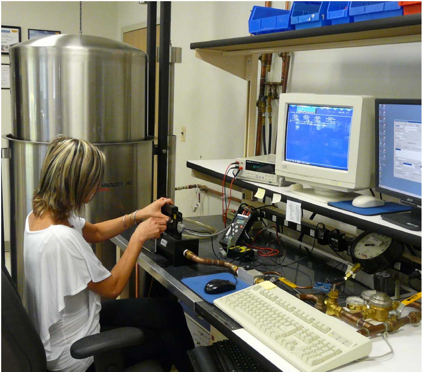
Bell prover used by technician in calibrating high flow capacity flow meter.
