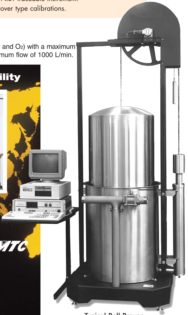
Typical Bell Prover used for NIST traceable calibrations
